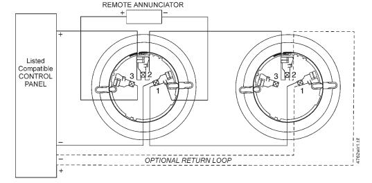
Wiring Diagram (standard base)
