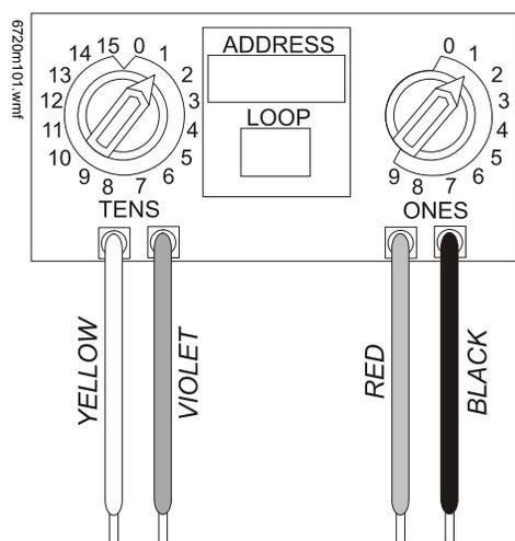
The NMM-100P(A) Mini Monitor Module can be installed in a single-gang junction directly behind the monitored unit. Its small size and light weight allow it to be installed without rigid mounting. The NMM-100P(A) is intended for use in intelligent, two-wire systems where the individual address of each module is selected using rotary switches. It provides a two-wire initiating device circuit for normally-open-contact fire alarm and security devices. NMM-100P(A)
