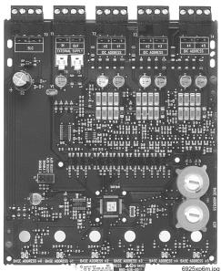
Maximum IDC wiring resistance: 25 ohms.
