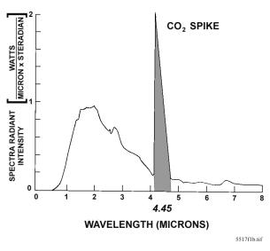
Figure 1 Spectral Sensitivity Range for Hydrocarbon Fires
