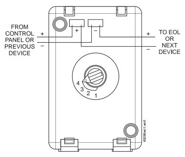
NOTE: SHOWN WITH CONTROL PANEL IN ALARM. PANEL POLARITY REVERSED IN SUPERVISORY CONDITION.
