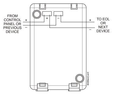
NOTE: SHOWN WITH CONTROL PANEL IN ALARM. PANEL POLARITY REVERSED IN SUPERVISORY CONDITION.
