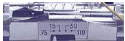
Multi-Candela Indicator(bottom of Strobe Lens)
