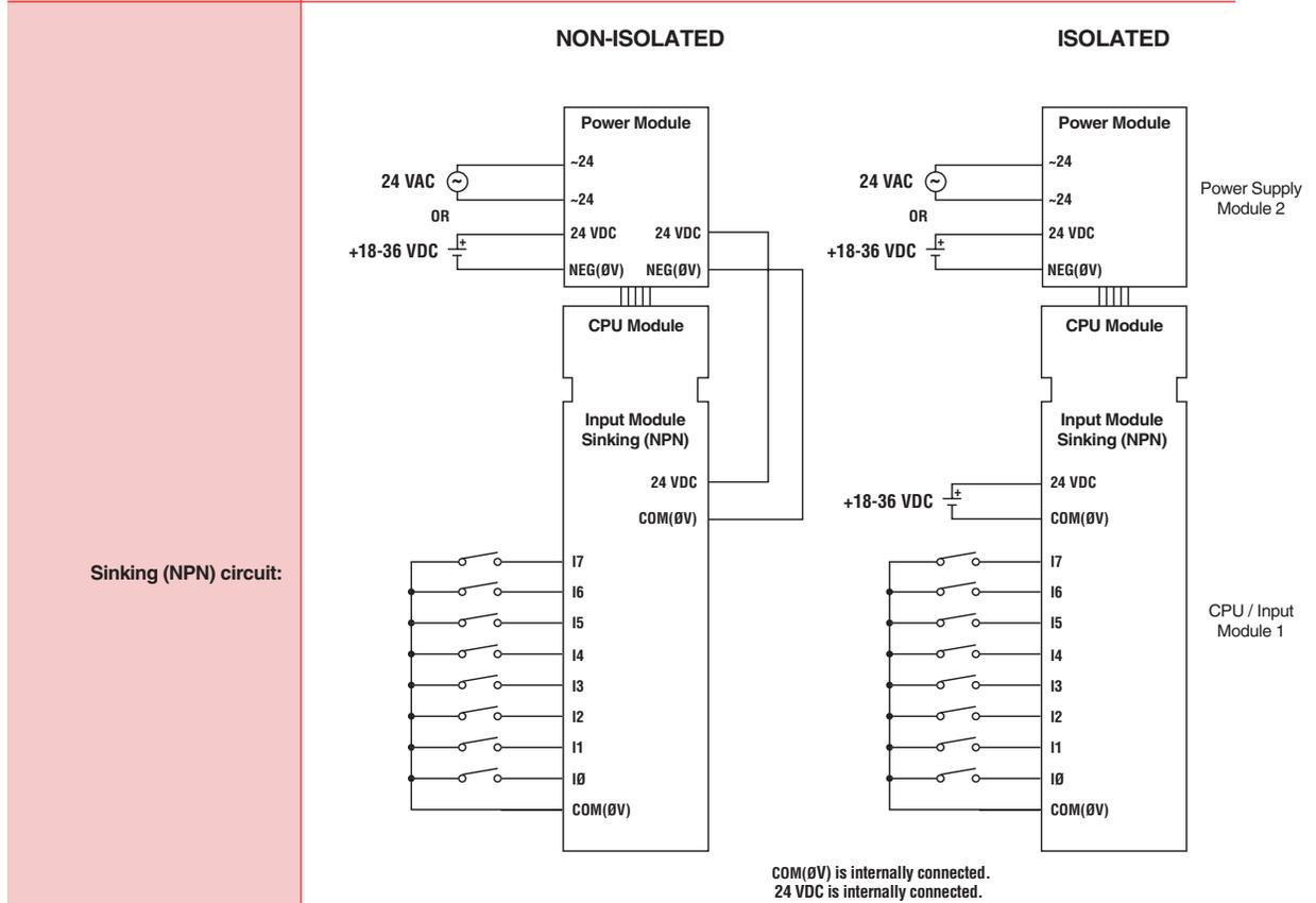
NOTE: All Input Modules are internally fused. Also, the Power Module is internally fused.
