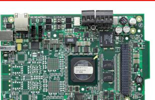
HS-NCM-MF: High-Speed Network Communications Module, fiber-optic cable interface (multi-mode).
