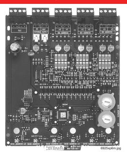
Maximum SLC wiring resistance: 40 or 50 ohms, panel dependent.
