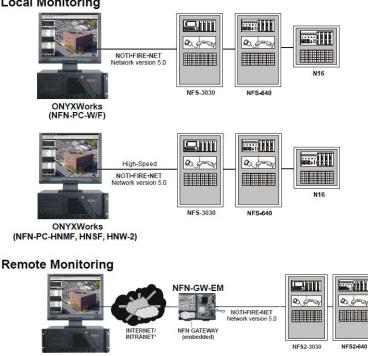
\* A UL Listed ethernet (TCP/IP) switch is required between a shared-IP network and the ONYXWORKS equipment
